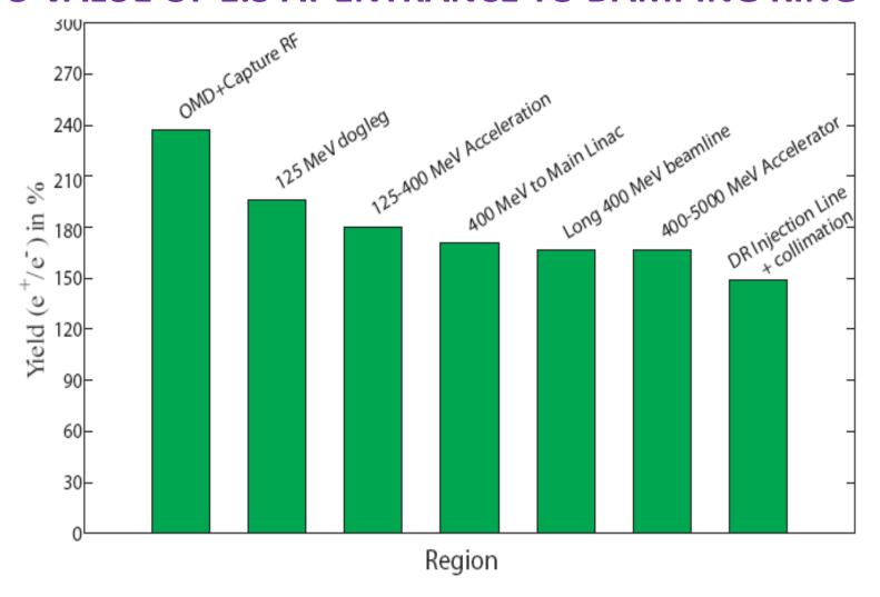
2.3-5. Positron yield in various parts of the Positron Source.
