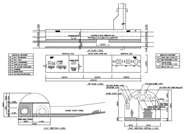
FIGURE 5.3-1. Detail of an access ramp for the Asian Sample Site.
