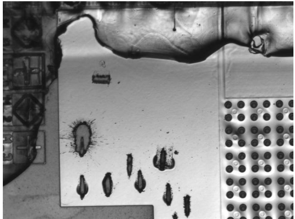
HV connection pad with prints of several attempts to bond them
