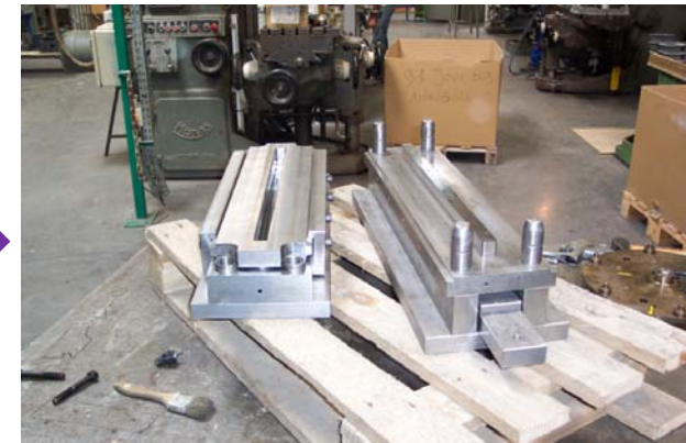
Mould delivered, ready to mould HexMC & SMC Carbon rails on a 80T heating press
