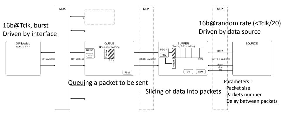
Two levels of buffers Modular design with similar interfaces Handshake protocols, optional MUXs Random data source to perform system tests
