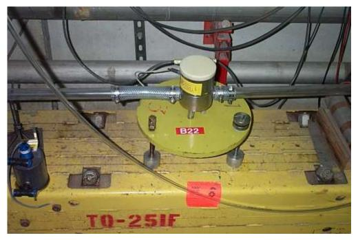
Fig.35. HLS probe on Tevatron accelerator focusing magnet.
