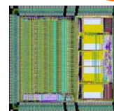
HARDROC Digital HCAL (RPC, \mu megas or GEMs) 64 ch. 16mm 2 Sept 06
