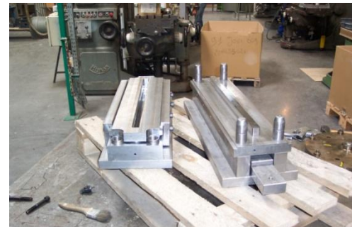
Mould for HexMC & SMC Carbon rails on a 80T heating press
