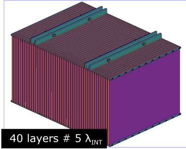
Eve of construction of 40 GRPC layers Large scale beam test in 2011 - Vital for Calice input to DBD 1m<sup>3</sup> stack can/will be partially equipped with Micromegas
