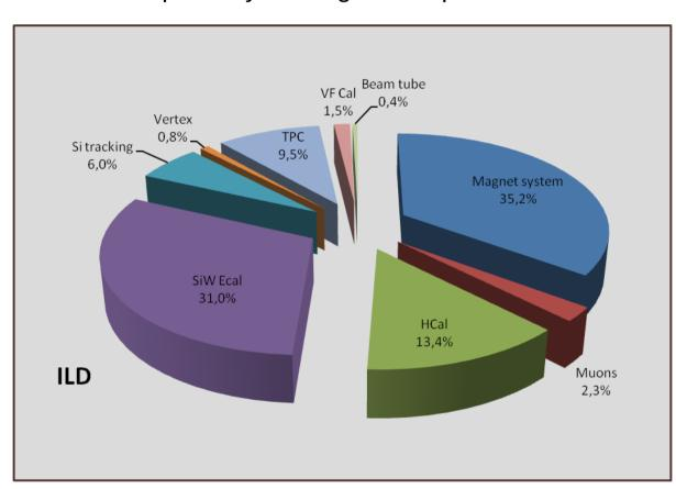
The cost is the cost for construction, R&D is not taken into account except specific R&D for transferring to industry.
