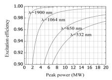
Required peak laser power for excitation of the n=2 level of hydrogen for different laser wavelengths
