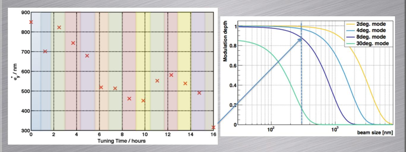
• Experience of application of tuning knobs during May running period at ATF2 with 10X nominal  $\beta^*$  optics (expected beam size ~150nm).
