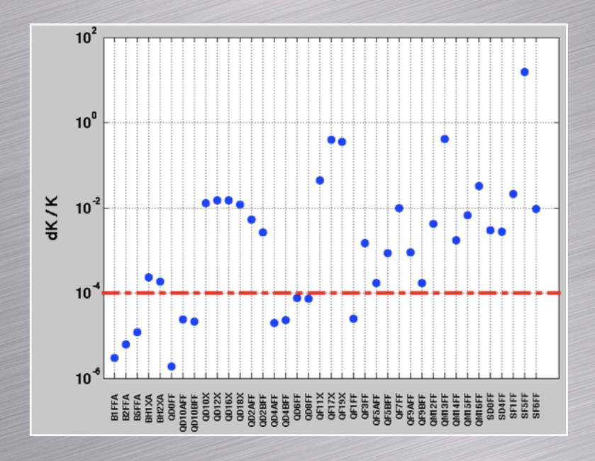
Relative setting error of magnets to produce an increase in vertical spot size at IP of 1nm.
