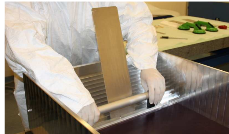
6 The alveolar layer is inserted in the mould with steel calibration foils
