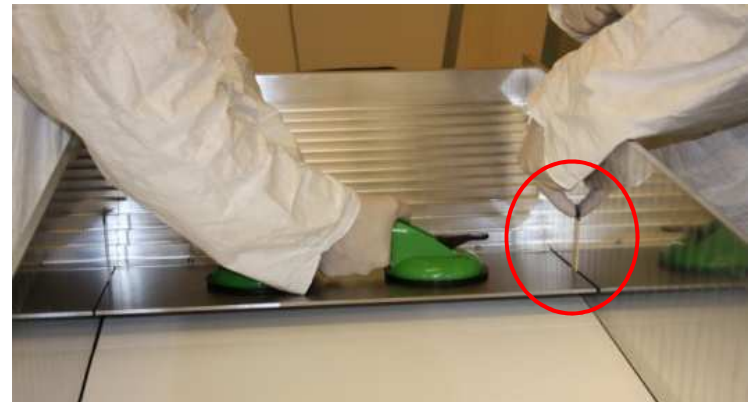
8 The tungsten plates are positioned precisely in the mould
