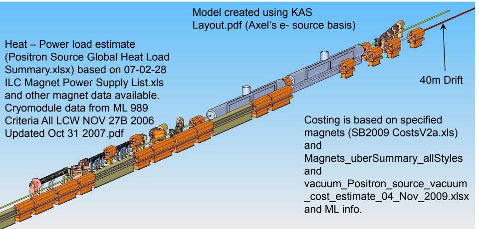
The AUX source is at this moment in time not much more than an artists impression. The lattice needs to be designed. It is feasible to utilise the photon vacuum vessel and the distance to the target needs to be defined.
