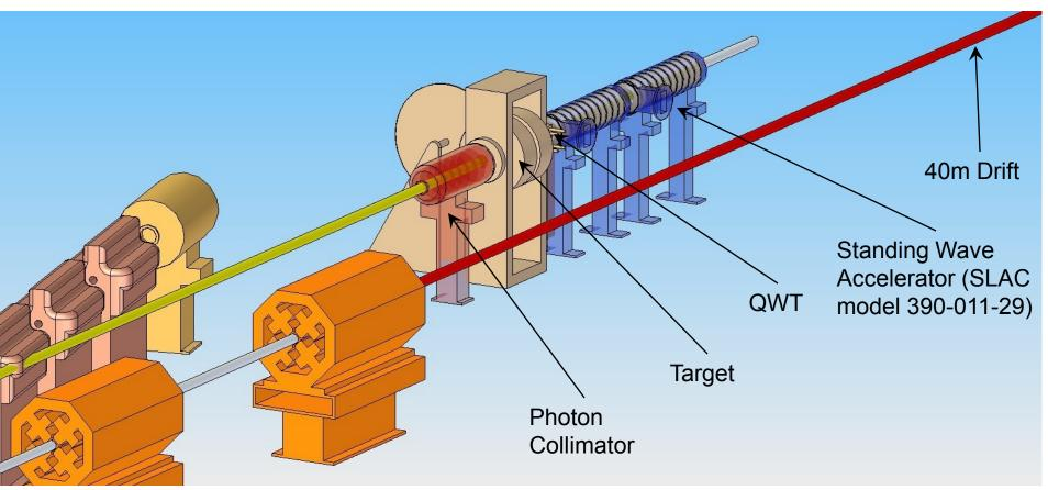
The Target Area has seen a lot of work during Positron Source workshops. The remote handling enclosure is not shown. The target requires a redesign to cater for the AUX source. Latest workshop info: <a href="http://indico.desy.de/conferenceOtherViews.py?view=standard&confld=3061">http://indico.desy.de/conferenceOtherViews.py?view=standard&confld=3061</a>
