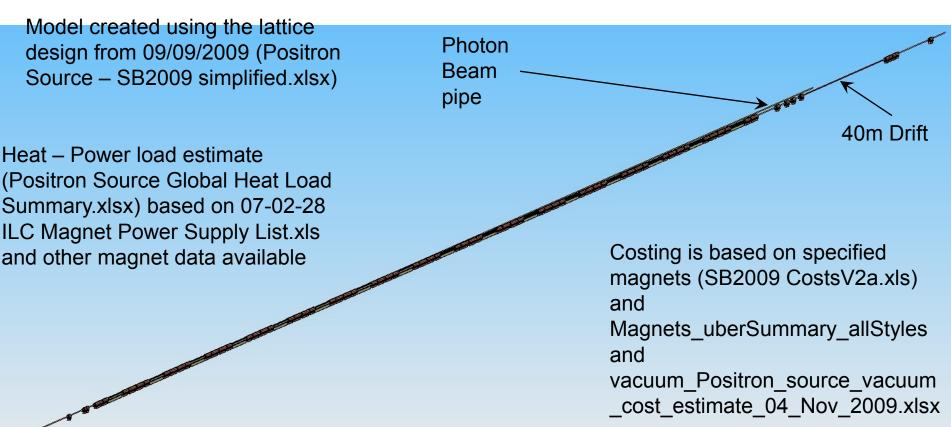
The dogleg provides a 1.5m beam offset. For the 10Hz low energy operation this must be revised. An Additional beam line is required and a 5Hz switching magnet. See 10HZ Low Energy Operation.pptx
