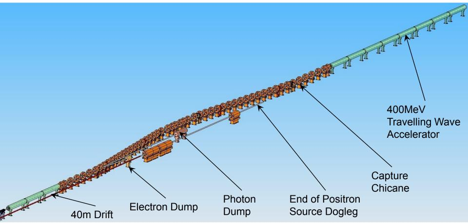
An additional Electron Dump is required due to the AUX source. The lattice needs to be designed as the illustration is a re-arrangement of the RDR layout (400 MeV in middle of chicane).
