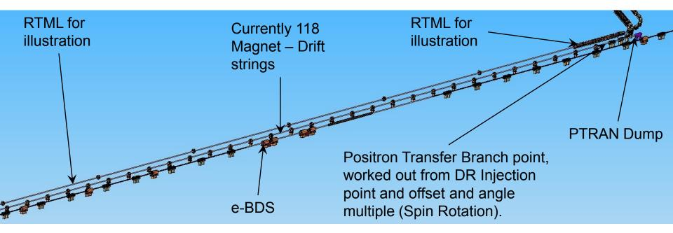
The lattice needs to be designed. Depending on the 5GeV Booster location, it is envisaged to have 118 magnet – drift strings.
