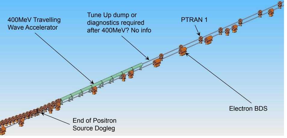
Again, this area is a best guess as far as CAD is concerned. The Positron Transfer (PTRAN1) is the same as the RDR where a Quad is followed by a drift. Lattice needs to be designed.
