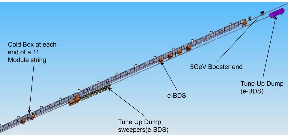
The lattice needs to be designed. The 5GeV Booster section can still move up or down the beam line (PTRAN). Currently shown just upstream of e-BDS Tune up dump for radiation and CF&S reasons.
