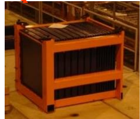
Scint. Strips-Fe Tail Catcher & Muon Tracker 5 \times 100 \text{ cm}^2 strips \sim 5 \lambda in 16 layer
