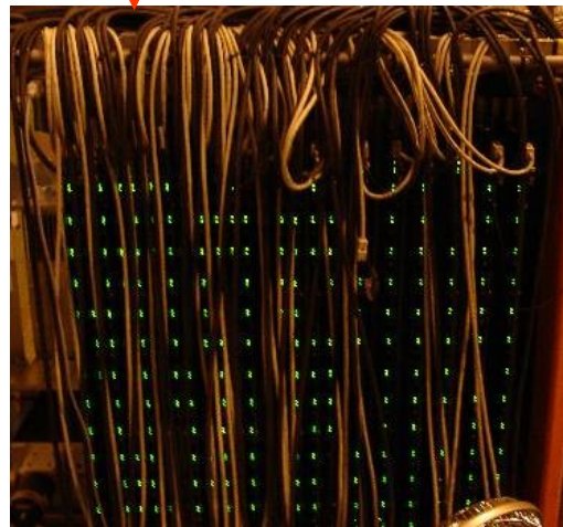
Scint. Tiles-Fe hadronic calor. 3 \times 3 \text{ cm}^2 lateral segmentation \sim 0.1 \lambda/\text{layer} , 38 layers
