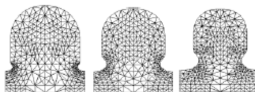
Figure 4. Profiles of the first, middle and last cell for 4.3m 3\pi/4 Mode TW structures.
