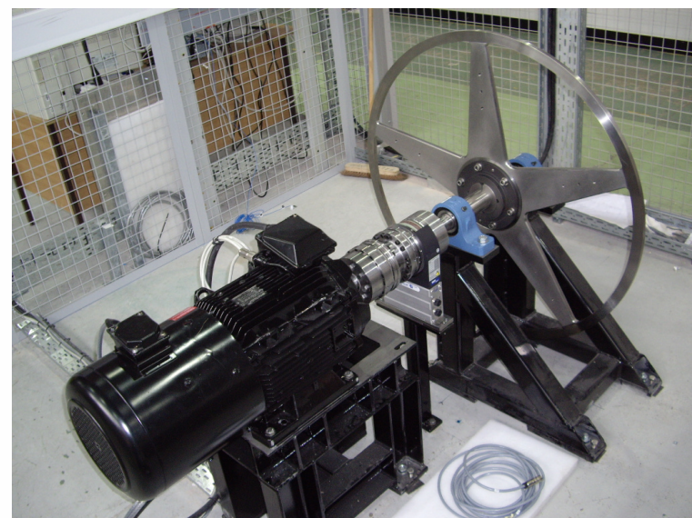
Daresbury Prototype Target wheel Solid Ti - No cooling
