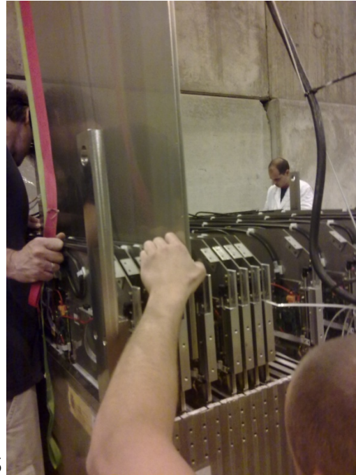
Instrument stainless steel stack with RPCs for June 2011 TB
