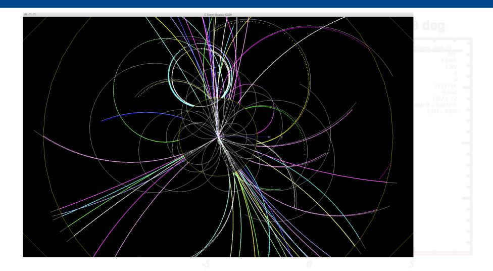
ttbar event @ 500 GeV reconstructed using Clupatra and SiliconTracking\_MarlinTrk then combined into full tracks using FullLDCTracking\_MarlinTrk pull Omega
