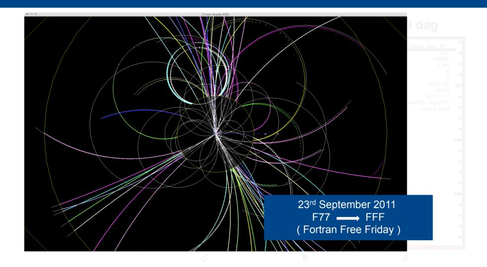
ttbar event @ 500 GeV reconstructed using Clupatra and SiliconTracking\_MarlinTrk then combined into full tracks using FullLDCTracking\_MarlinTrk
