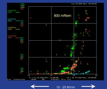
Maximum X-rays at opposite end of Cryomodule
