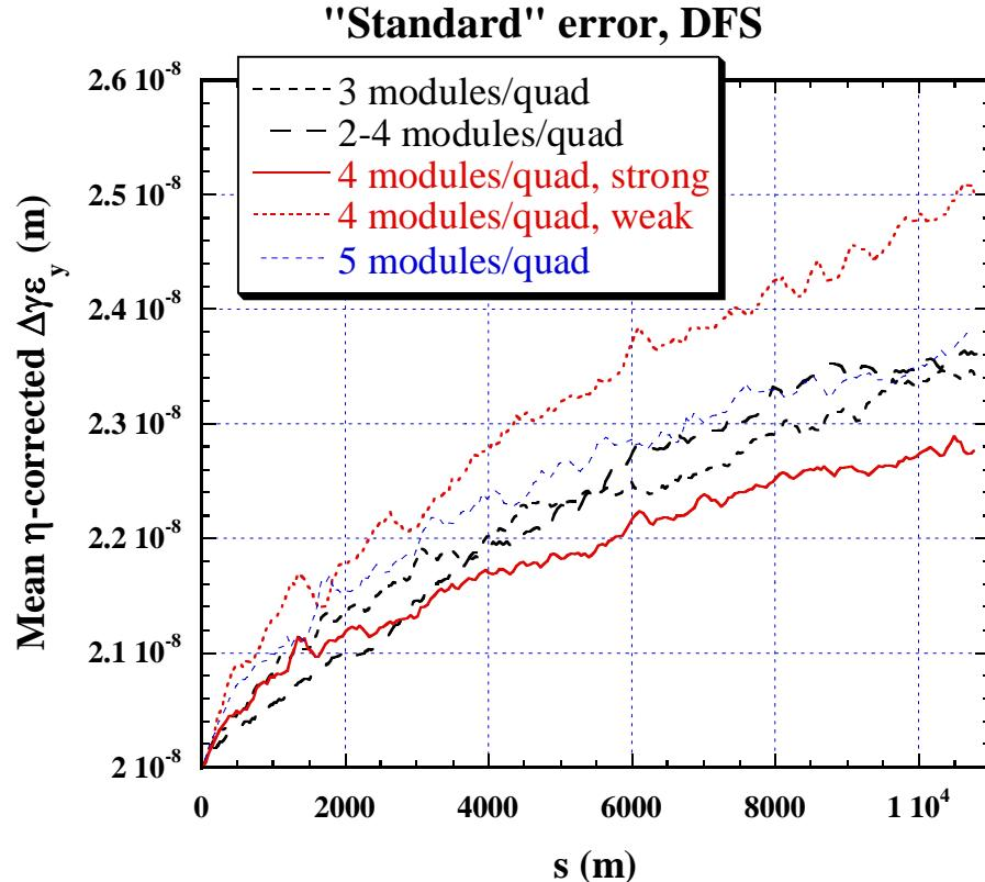
Errors: Quad offset 360 um, Cavity offset 640 um, BPM offset 360 um
