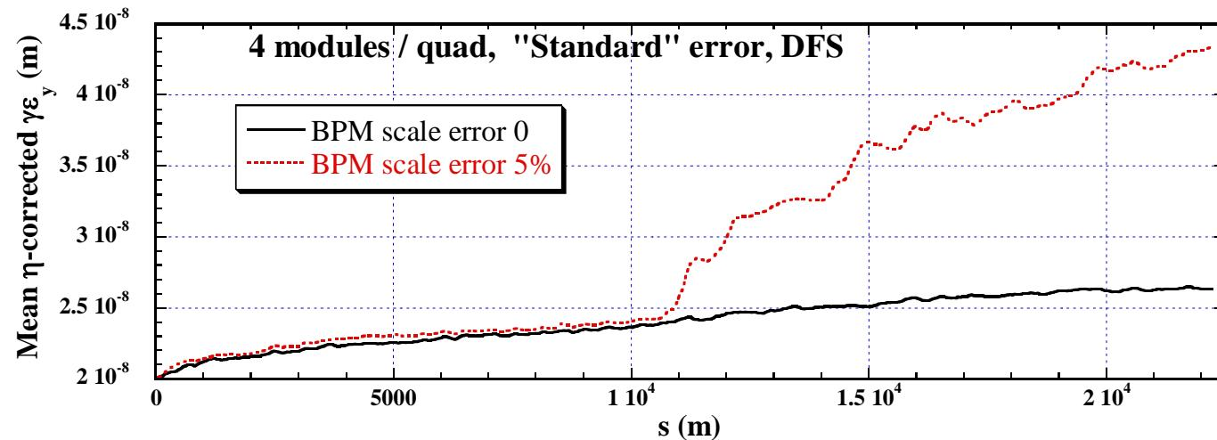
Errors: Quad offset 360 um, Cavity offset 640 um, BPM offset 360 um
