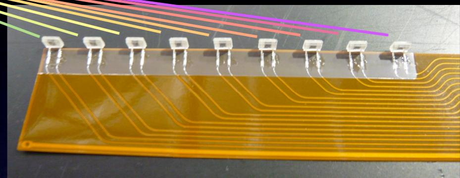
Holding W absorber (3.5 mmT) behind the strip scintillators
