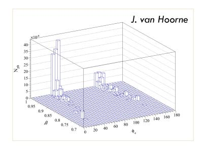
Transmitted photon distribution, normalized to one lost beam electron, for single loss at 2.4 GeV in the DB.
