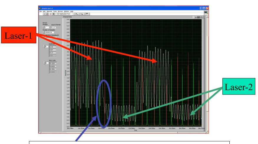
Chopper edge effects and low photodiode duty cycle per laser complicate measurement.
