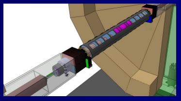
Carbon tube made with pipes for laser beams (higher stiffness)
