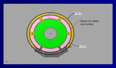
The electronic channels of LumiCal will be read in digital form to the DAQ placed  $\sim \! 10$  m far from the detector outside the ILD. The cooper LVDS TP cables will go from each half plane of LumiCal around the barrel to the back side of each LumiCal where Data Concentrator will be placed. From Data Concentrator we foresee optical links to the DAQ. The fibre optics cables will go over LHCal and inside the square support tube (near QD $_0$  magnet) outside the ILD detector.
