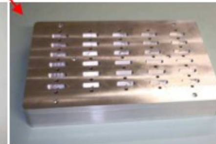
Joints production : 180/180 joints ready Design and construction of 2 moulds according to lower and upper parts
