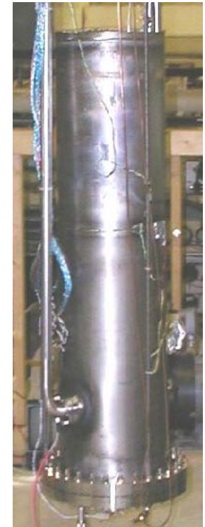
80.5 MHz Quarter-Wave resonator
