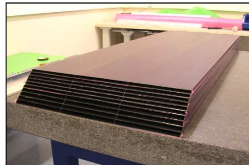
All the 15 structures are been moulded The production of one layer with the FBG is now finish.
