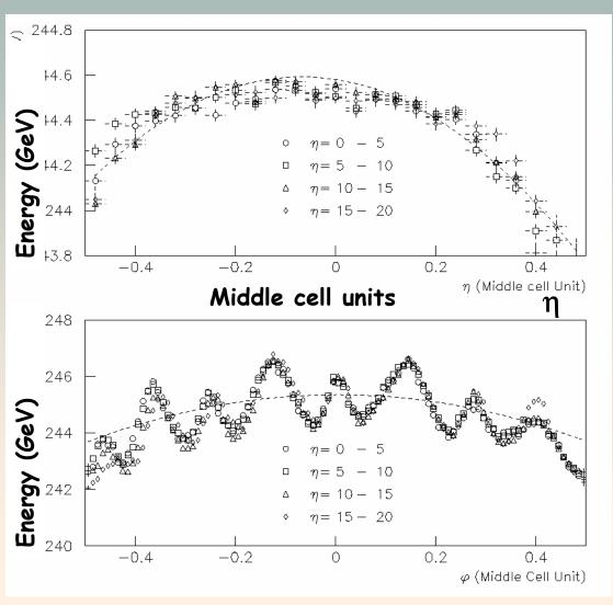
Universality of corrections which are determined on Data in the barrel, the same for all modules.
