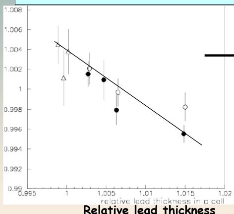
1% Pb variation  $\rightarrow$  0.6% drop in response Measured dispersion  $\sigma$  = 9  $\mu$ m (calo) Translates to < 2 % effect on constant term
