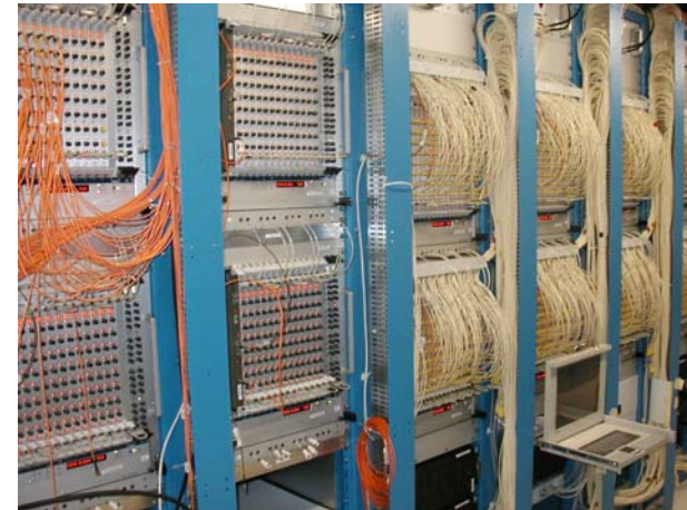
Racks and crates for ROD system, powered, tested with the Injector. Connection with FEBs in progress.
