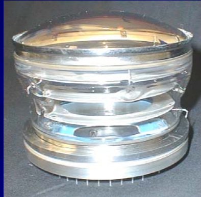
HPD tube manufactured at CERN: 2048 channels
