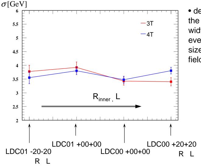
• dependence of the reconstructed width of Z pole events on detector size and magnetic field.
