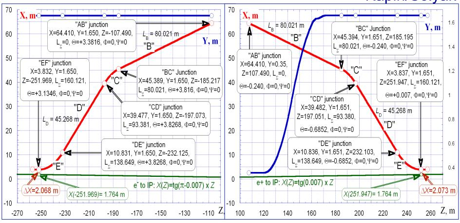
Good symmetry in X0Z plane between PRTL and ERTL (while the same  $L_{\Sigma}$ ) Good coincidence between the "ideal" layout and the lattice survey
