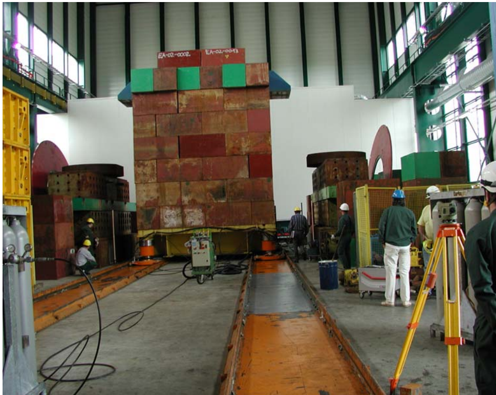
Figure 1. Insertion of the 1000 tons on the plug – 15/05/2006
