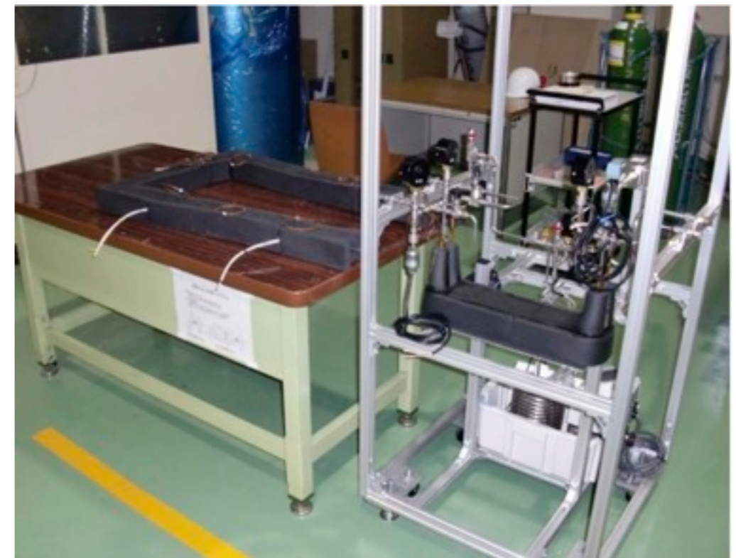
First CO 2 cooling system constructed in KEK
