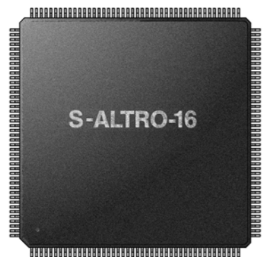
Wire bonding package 24mm x 24mm x 1.4mm
