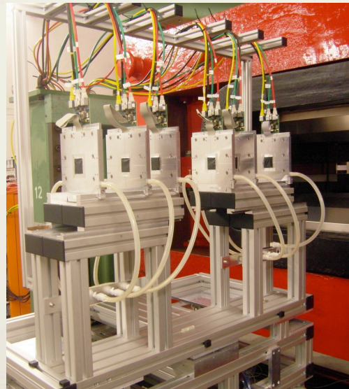
Beam telescope in the CERN and DESY test beam lines based on the MIMOSA-26 pixel sensors. Image: DESY
