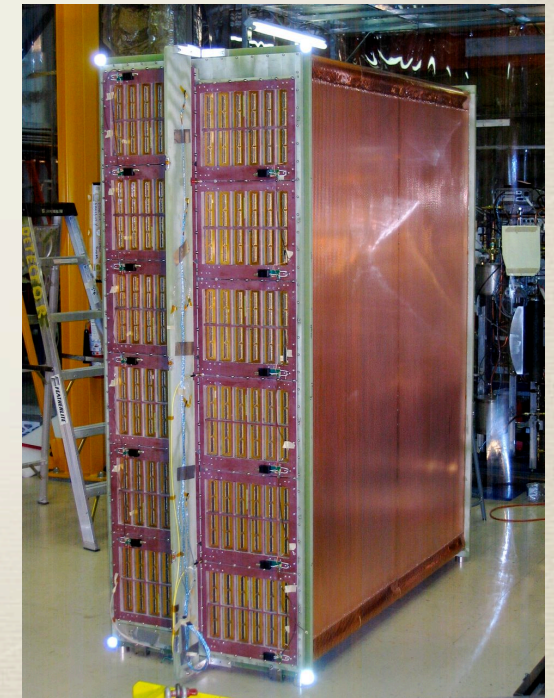
MicoMegas-based time projection chamber for the T2K experiment in Japan, based on ILC detector R&D. Image: T2K
