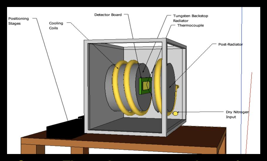
Status: Thermal prototype under testing at SCIPP
