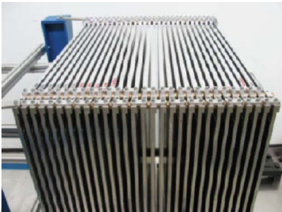
tail catcher: installed for higher energy program
