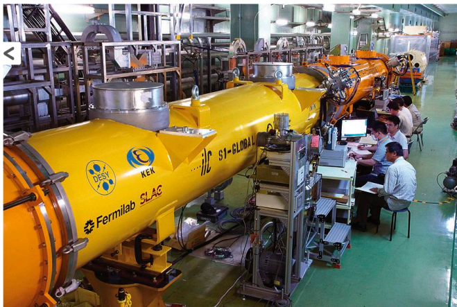
At KEK in Japan, accelerator experts test advanced superconducting radiofrequency technology, under development for the proposed International Linear Collider. The technology combines efforts and components from DESY (Germany), INFN Milano-LASA (Italy), KEK (Japan), Fermilab and SLAC (US).
