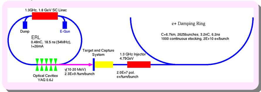
For Linac Compton Scheme, we can reuse 6GeV e-Linac with  $CO_2$  laser cavity system. Also, the 6GeV Linac has to accelerate 10nC bunched beam with 132 bunches/pulse.
