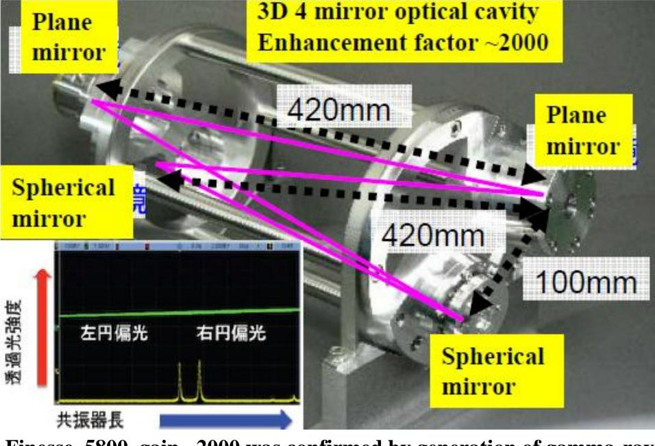
Finesse 5800, gain ~2000 was confirmed by generation of gamma-ray last year. Also, laser waist size was less than 15 $\mu$ m.
