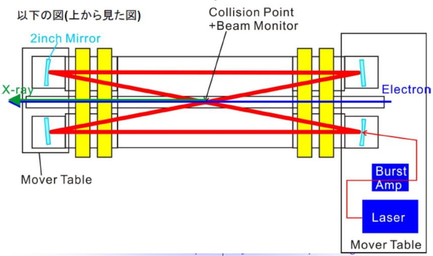
Change to head collision scheme to get another enhancement of 5 and to increase laser pulse duration ~30ps.
