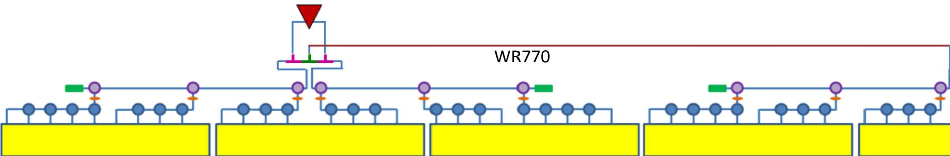
For low power **Kamaboko** Tunnel option, one klystron powers 1 ½ rf units or 4 ½ cryomodules (39 cavities).
