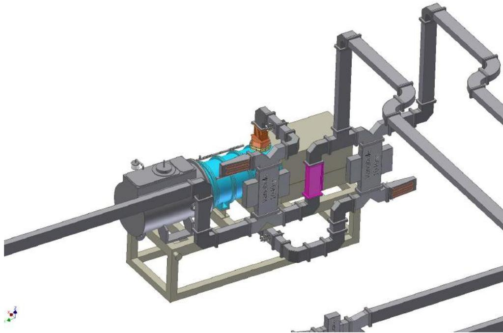
Jog in feedthrough waveguides to prevent radiation leakage.
