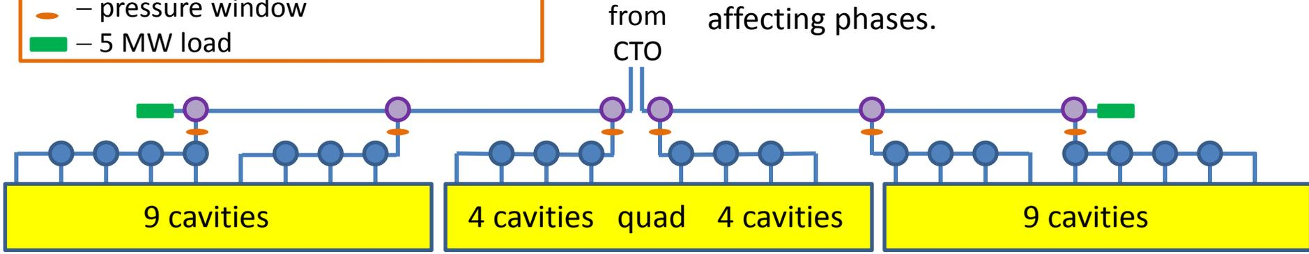
phase shifter on each feed, as well as isolator, bi-directional coupler, and flex guide.
