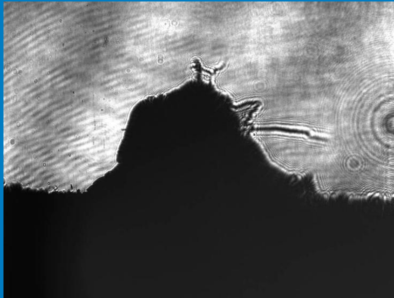
OTR screen illuminated with alignment laser showing notch
