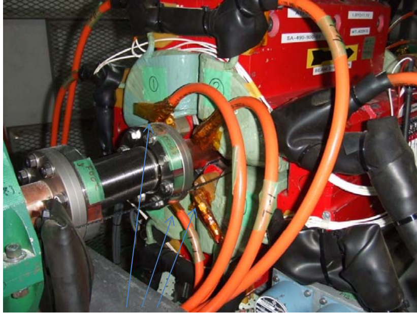
Connector of cooling water (magnetic material)
