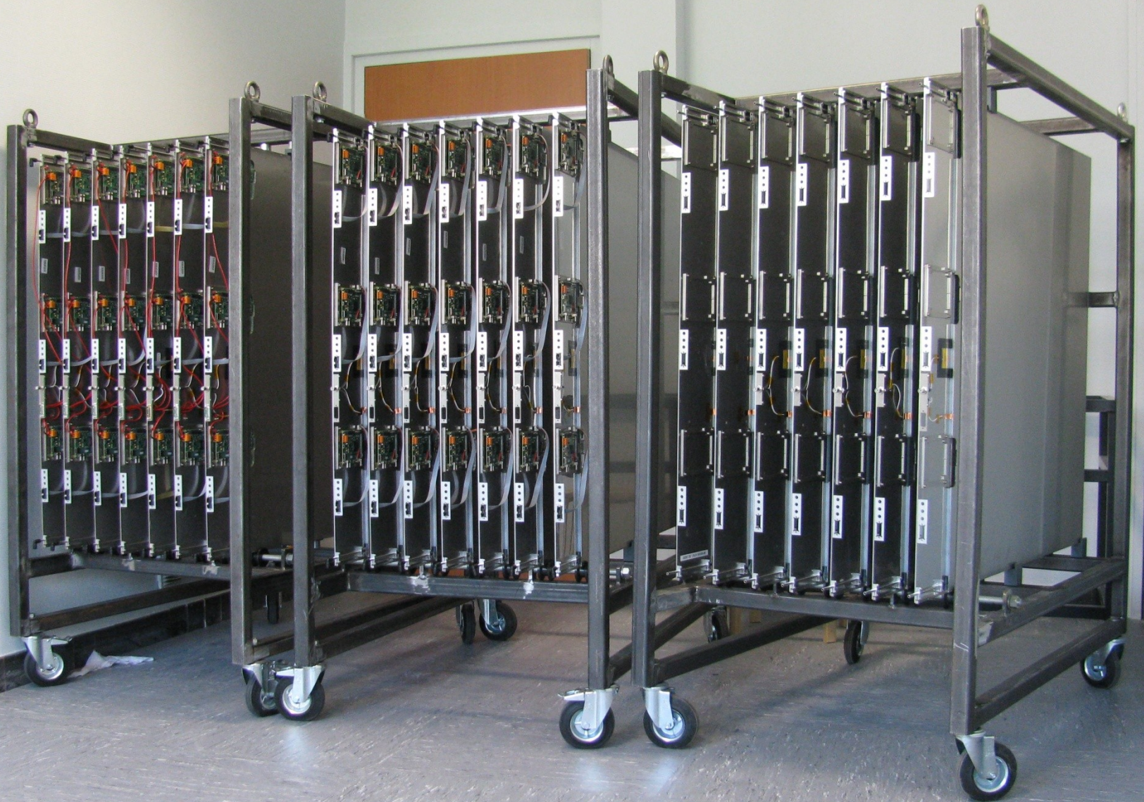
50 GRPC Chambers have been built to be used in the SDHCAL prototype
