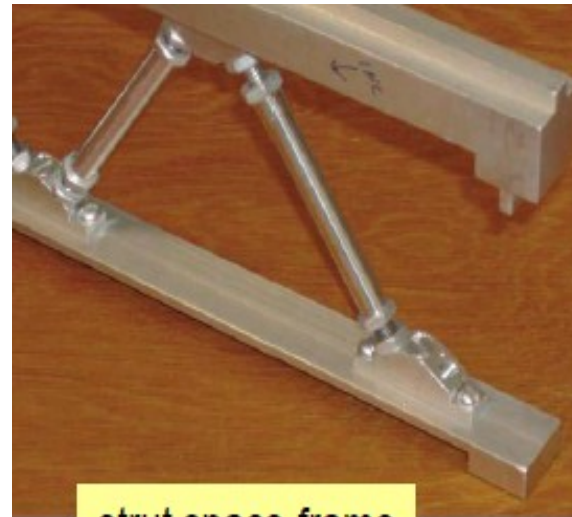
strut space-frame test structure
