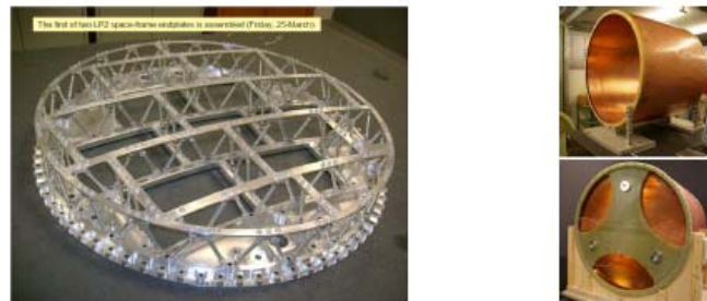
Figure 7: LP prototype of the advanced endplate (left) and the fieldcage (right).
