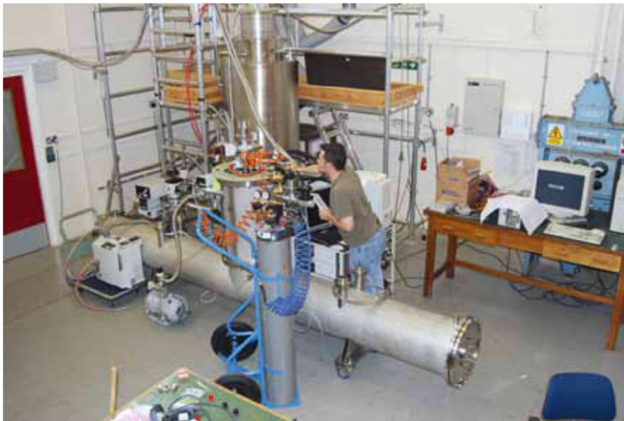
Figure 5.3.2.2 The 4-m cryostat prototype superconducting helical undulator under test at Rutherford Appleton Laboratory.
