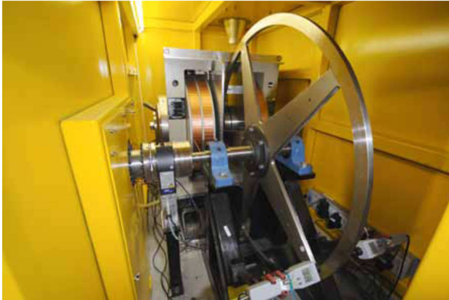
Figure 5.3.3-1 Prototype rotating target setup for eddy current tests at Daresbury Lab. Copyright STFC.
