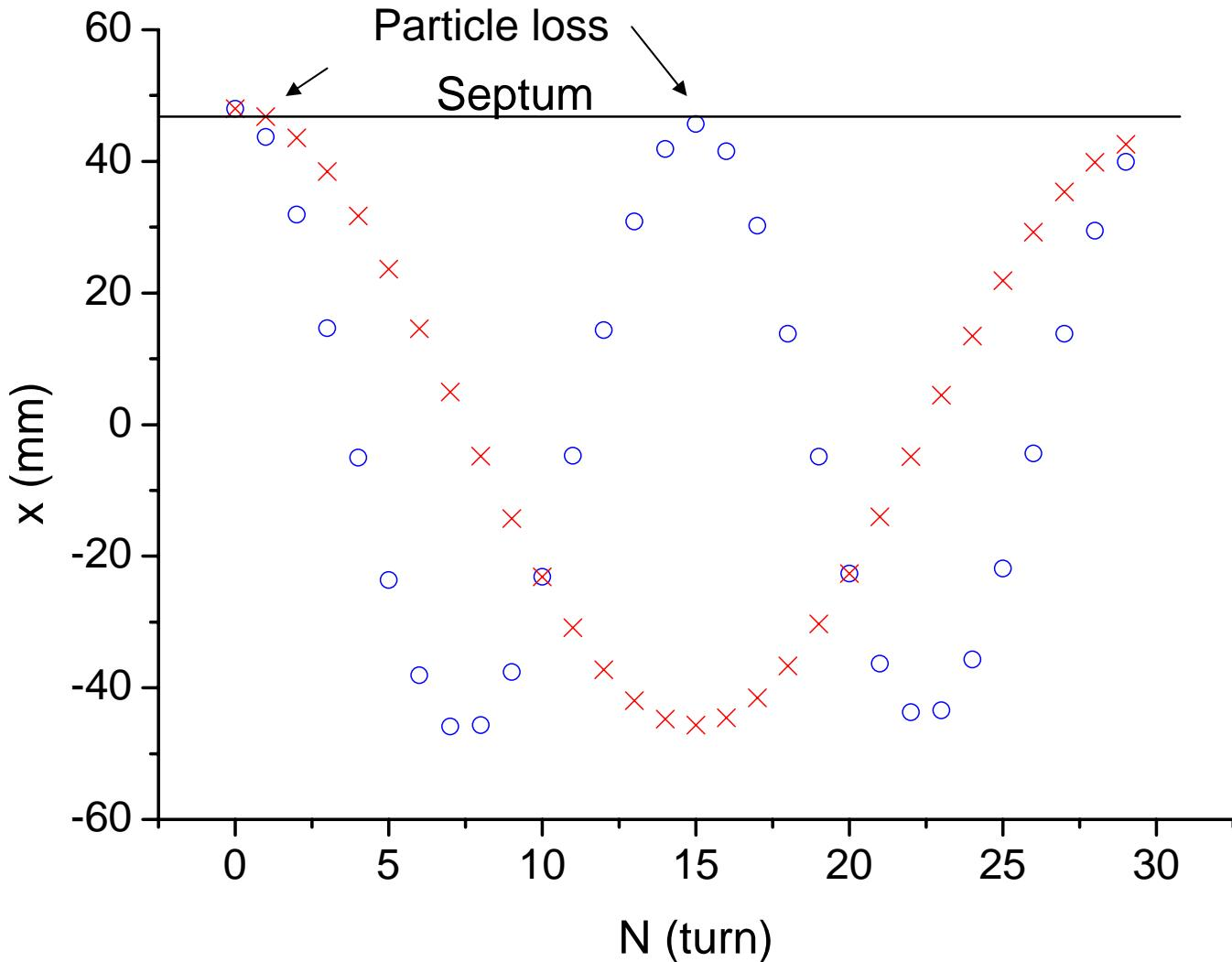
**Positions of equilibrium orbit. Dispersion at injection azimuth  $\eta=0.6$  m, momentum deviation  $\Delta p/p=8\%$ , synchrotron frequency  $Q_s = 1/15; 1/30$ . Ring circumference  $C=100$  m, synchrotron damping  $\tau_s=100$   $\mu$ s (333 turns)**
