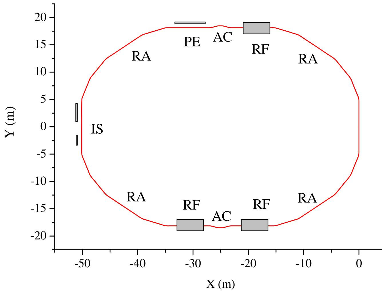
**Ring layout. Energy  $E_0=3.5 \text{ GeV}$ , circumference  $C \approx 144 \text{ m}$ , bend.field  $B=6 \text{ T}$ , energy losses  $\Delta E \approx 9.4 \text{ MeV} / \text{turn}$ , synchrotron damping time  $\tau_s \approx 250 \mu\text{s}$ .**
