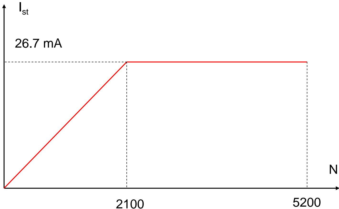
$$N_{pb} = 4*10^9/3 \Rightarrow \langle I_{st} \rangle = 0.22 \text{ A}; N_{bb} = 8 \Rightarrow \langle I_{st} \rangle = 27 \text{ mA};$$
