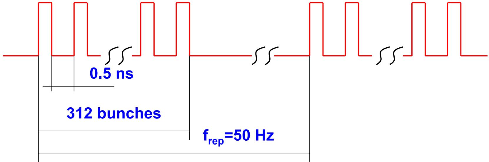
$$N_{pb} = 4 \times 10^9 \Rightarrow Q_b \approx 0.64 \text{ nC} \Rightarrow \langle I_{stor} \rangle = 0.64 \text{ A},$$
