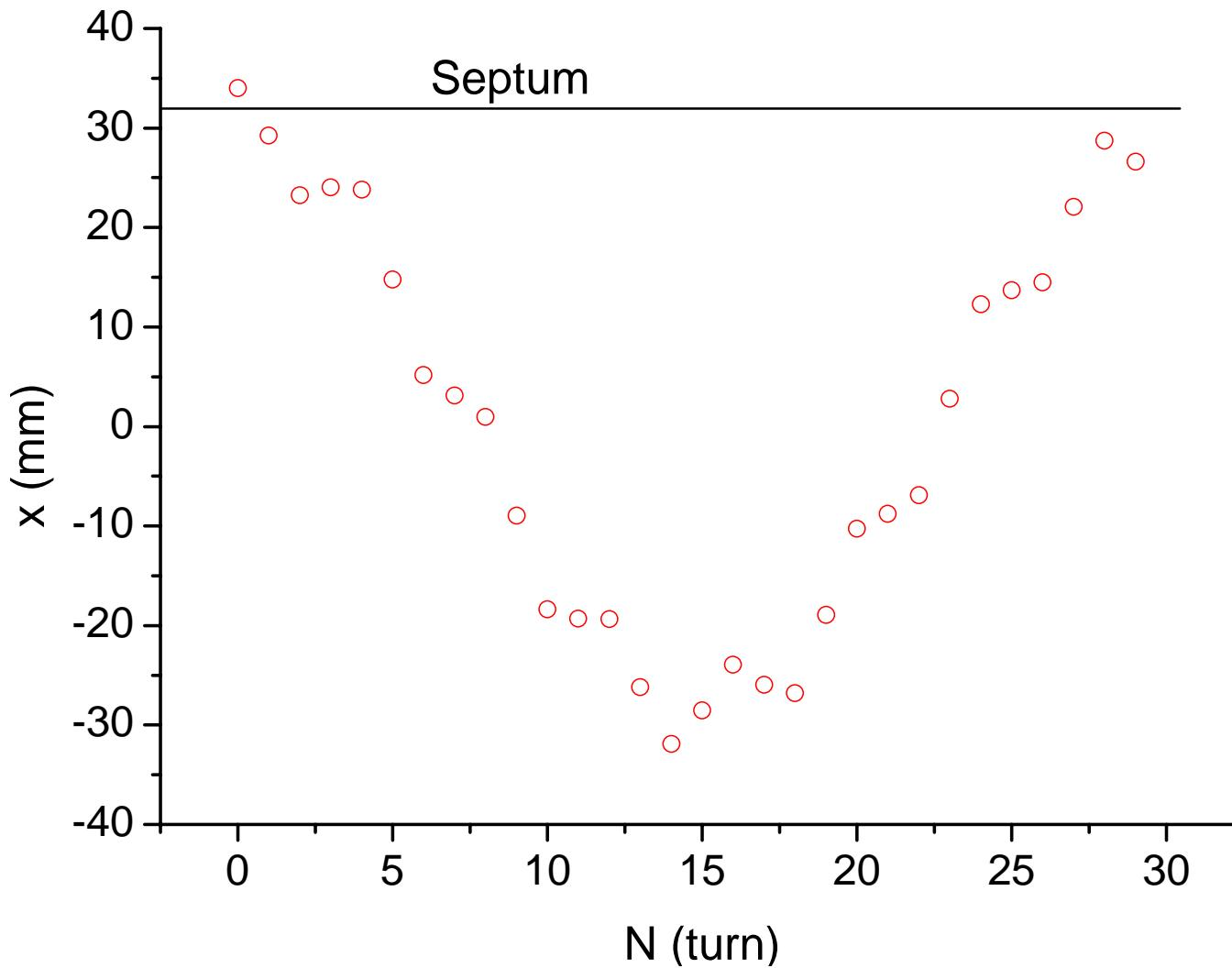
**Resultant motion of injected particle. Dispersion at injection azimuth
