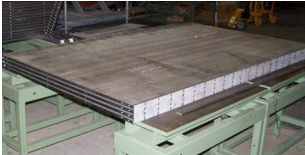
2160 mm sub-module plates after roller leveling max 1 mm deviation
