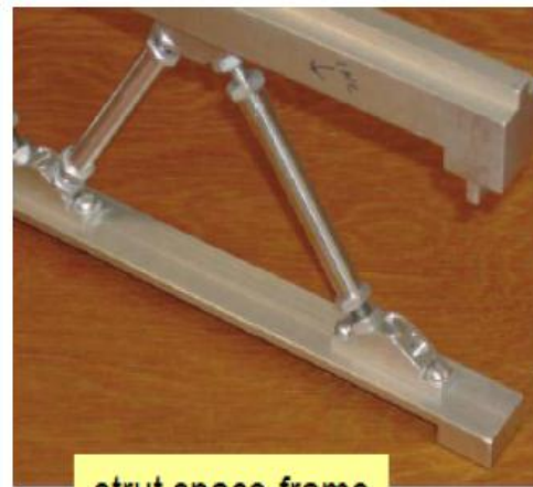
strut space-frame test structure
